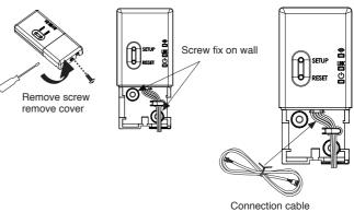
3. Insert lead wire in to unit and connect Communication cable.
