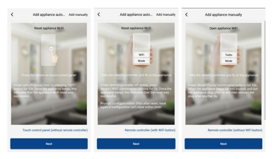
Reset the air conditioner (refer to the operation instructions in APP interface) and click "Next" to add home appliance automatically (Wi-Fi password shall be input). Or after setting and energizing the air conditioner, click "Add appliance manually" at the right upper corner to select the wireless network for controlling the device. Then confirm family Wi-Fi and arrange configuration.
